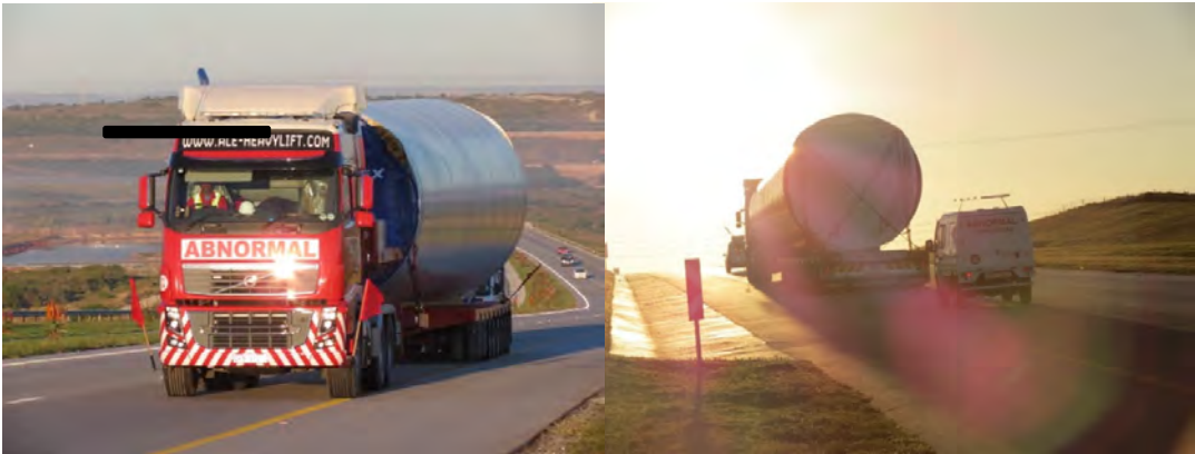
Figure 2-4: Example – Transportation of Tower Sections
